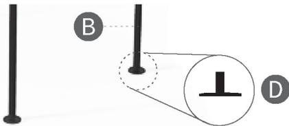
**EN** Screw feet to bottom of legs for leveling the planter.
