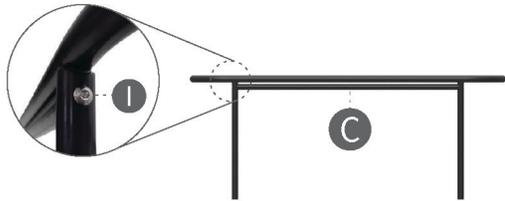
**EN** Insert tension bar between openings at top of legs and fasten securely with **flat head screws**. (Make sure screw is being installed from side with indentation on tube).
