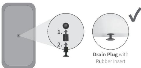
**EN** Place rubber tube inside the planter hole. Then introduce the grey plug. Make sure to push until grey plug has entered all the way.
